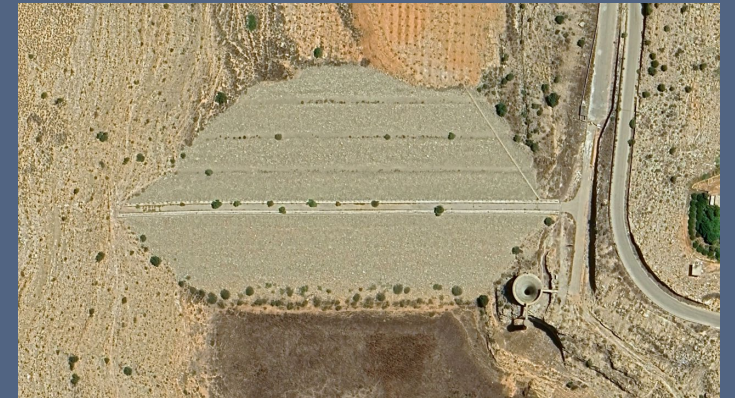
Abu Mansour dam H_{max} 73m (48m) Vol 23.7 Mm 3
